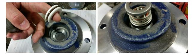
Then place the ceramic half of the seal in the housing, use soap to lubricate and press in to the bottom. The groove side will face down or towards the motor side.
