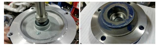
Now with the aux shaft attached, place the pump housing (282-6307) to the motor.
