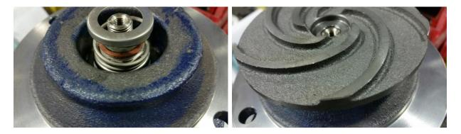
Place the black graphite half on the shaft and press until it is touching the white ceramic half. Use soap to lubricate the inside of the black rubber half. Be careful with this operation, the ceramic portion is glass and can break when blows are laid against parts of the pump.
