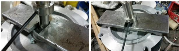
In the field, a gauge can be made by cutting a template from cardboard and use it to mark the shaft.
