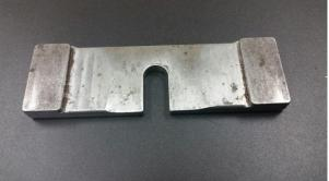
At the factory, a machined gauge is used to set up the distance.
