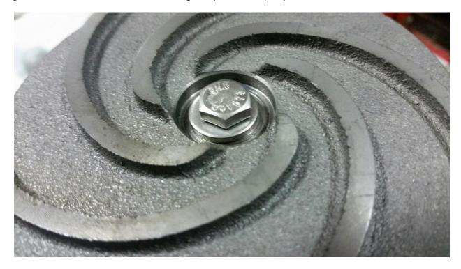
Then twist the impeller to the right as looking at it from this picture, when it seats hand tight, place the secure bolt and washer (098-1443, 098-2413) in the end of the shaft and tighten.
